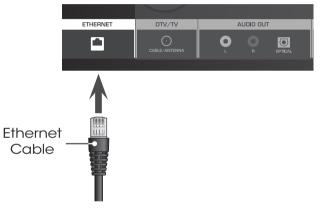
If you have a high-speed Internet connection, connect an Ethernet cable from your modem/ router to the back of the TV as shown.
